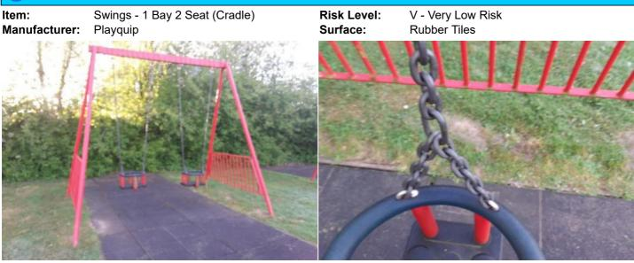
**Finding:** The surfacing width under each seat is less than 1.75 metres and fails the requirements of BS EN 1176 Part 2
