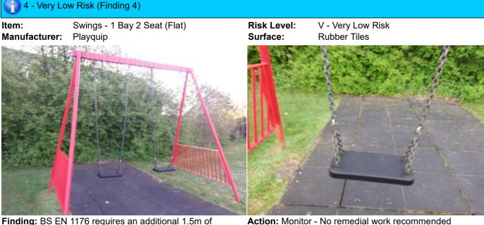
Finding: BS EN 1176 requires an additional 1.5m of unobstructed space at each end of the swing surfacing area. This is a relatively low risk finding and no remedial action is recommended at this point.
